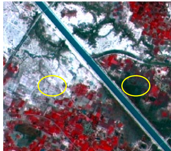
Waterlogging due to Canal Seepage
